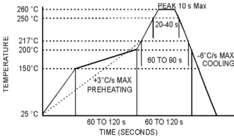
The device may be reflowed once. Reflowing upside down is not allowed. NO CLEAN assembly is recommended
